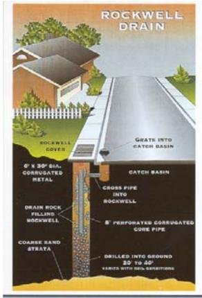
Modesto has two drainage systems—the sewers and the *storm drains*. The storm drain system was designed to prevent flooding by carrying excess rainwater away from city streets and out to our rivers by way of catch basins or drainage into our rockwell system.
